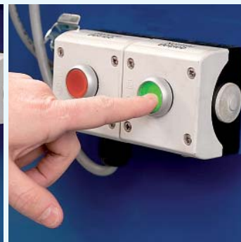
Pic. 3: Normal Operation is confirmed by push-button.
