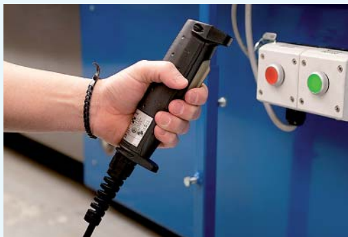
Pic. 2: The middle position of the manual control switch activates Service Operation.
